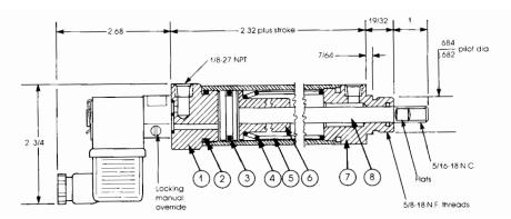
HOW TO ORDER: WHEN ORDERING PLEASE SPECIFY MODEL NO. – STROKE – PLAIN ROD END IF DESIRED – MOUNTING BRACKETS (IF REQUIRED) – VOLTAGE BORE SIZE 1-1/8" – MODEL NUMBER 6110501\*. SEE PAGES 6 & 7 FOR OPTION CODES AND ADDITIONAL ORDERING INFORMATION. \*SPECIFY STROKE LENGTH AND VOLTAGE. EXAMPLE 6110501-02.00 – 120VAC. FOR OPTIONAL TRUNNION MOUNT VERSION. CONSULT FACTORY.
